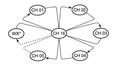
Priority scan searches through all tag channels in sequence while monitoring channel 16. When a signal is detected on channel 16, scan pauses until the signal disappears; when a signal is detected on a channel other than channel 16, scan becomes dualwatch until the signal disappears.
