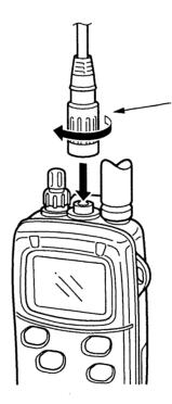
**CAUTION:** Attach the speaker-microphone's connector securely to prevent accidental dropping, or water intrusion in the connector.
